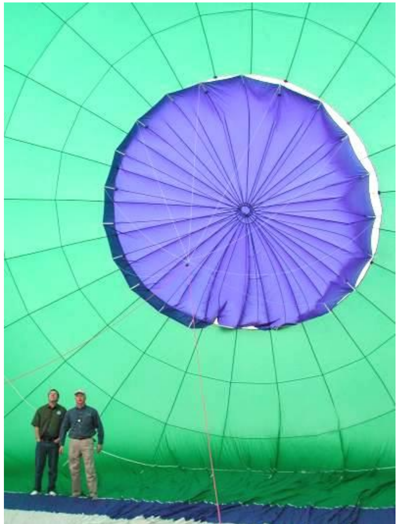
The parachute valve, from the inside of the balloon. A Kevlar cord runs from the valve at the top of the balloon, down to the basket, through the center of the envelope.
